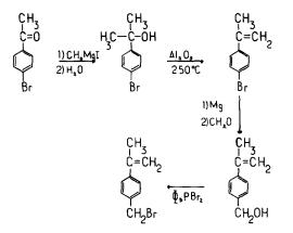
The overall yield with respect to p.bromoacetophenone is of the order of 40%. The pure p.bromomethyl- $\propto$ -methylstyrene is a white crystalline solid melting at 41°C. It was never described before, to our knowledge.
